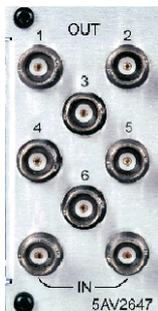
input is terminated in 75Ω either on the unit or at the end of any interconnecting cable. Ensure that all unused outputs are terminated in 75Ω.
