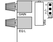
Front panel gain and equalisation controls are at unity gain and 0m equalisation when the knob pointers align with the panel marker. Turning the control clockwise increases, and anticlockwise decreases, the Gain and Equalisation respectively. Section 3.1 describes the alignment procedure using a Pulse & Bar test signal to equalise a signal.
